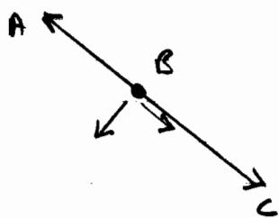
Resolving the weight of the box parallel and perpendicular to ABC, the perpendicular component could not be supported by the two strings.  $\therefore$  an impossible situation.
