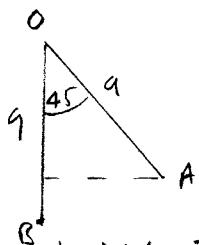
$$\text{Loss in height} = 9 - 9 \cos 45^\circ \\ = 2.636 \text{ m}$$
